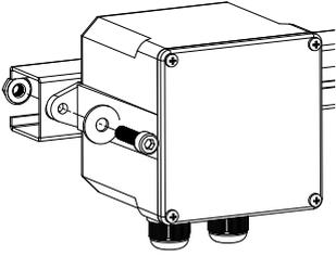
**Step 3. Connect the cables to the branch junction box**
