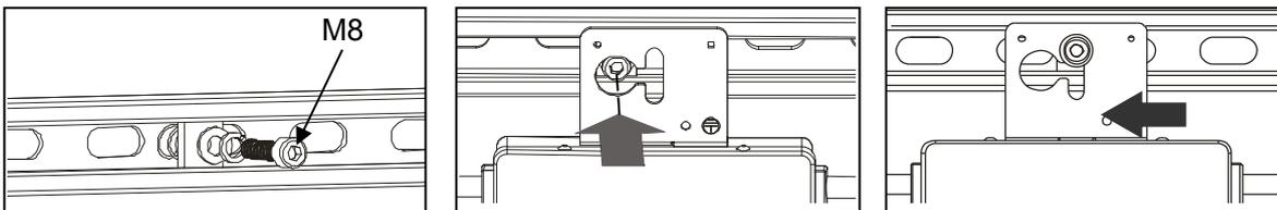
**Step 5.** Connect the APsystems Microinverter AC Cables
