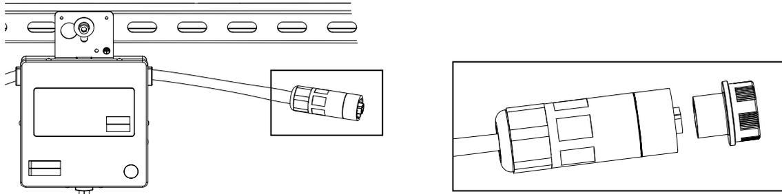
**Step 7. Place the PV modules and connecting each YC250 to the PV modules**
