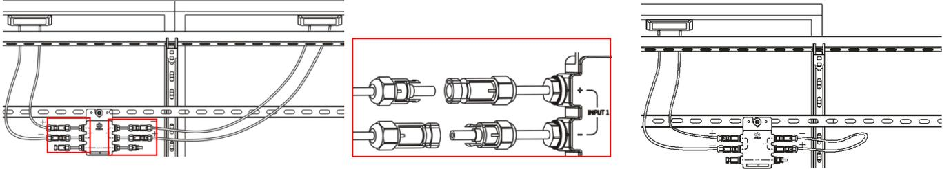
**WARNING:** Connect the PV module to the optimizer INPUT1 interface when the optimizer connects with one solar module, then connect DC Extension Cable to INPUT2 interface shorted.
